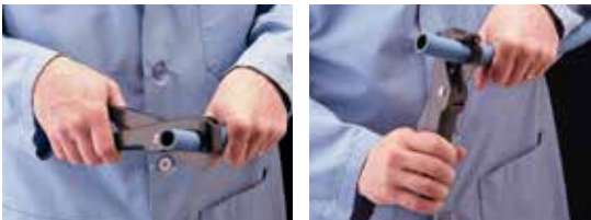
The rotating/rocking technique produces fast easy cuts.
