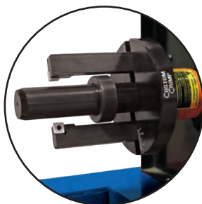
OD Skiving Tool & PTO Coupling: Long lasting carbide inserts have multiple cutting edges to eliminate sharpening and PTO Coupling for quick change tool.
