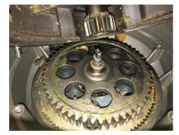
Robust materials are selected for loaded parts; for example, sintered alloy epicyclical gearing and cast-iron output drives.
