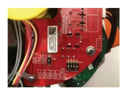
OM1: input/output module offers analog positioning control and position feedback, 4 additional SPST output contacts (configurable) independently settable at 10 points along the stroke, optional Bluetooth interface, information about loss of input signal and Bluetooth failure, and a local selector position alarm (with OM3 installed).
