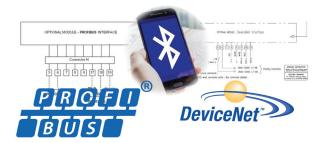
Simple connection to a bus system is possible with the optional OM9 (PROFIBUS DPV0/V1) and OM11 (DeviceNet) communication cards and setting all parameters via configuration software on a Bluetooth-enabled PC or PDA. Bluetooth is included as standard with the OM9 and OM11 cards.
