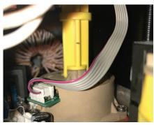
Absolute position sensor covers 110° of rotation, with travel endpoints set by the rotary switch (standard) or set non-intrusively (via optional Bluetooth).
