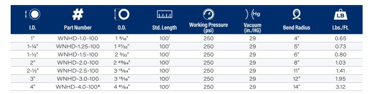
4" Balthazar HD uses a steel helix construction, is NOT crushproof
