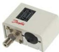
Danfoss KP pressure switches are used for regulating, monitoring and alarm systems in industrial applications. The KP series are suitable for gaseous media and air. They are fitted with a single-pole switch changeover (SPDT), and can control single-phase ac motors of up to 2 kW directly.
