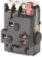
The thermal overload relays TI 9 C cover the range from 0.13 - 9.2 Amp. The phase failure function accelerates the trip function by three phase run if a phase drop-out occurs. This is particularly important for delta connected motors.
