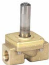
EV225B is a servo-operated 2/2-way solenoid valve for use in steam application. The design is based on a PTFE diaphragm concept, ensuring high reliable function even in connection with contaminated steam.
