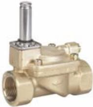
EV220B 15-50 is a universal indirect servo-operated 2/2-way solenoid valve program. Valve body in brass, dezincification resistant brass and stainless steel ensures that a broad variety of application can be covered. Built-in pilot filter as standard, adjustable closing time and enclosures up to IP67 ensures optimal performance even under critical working conditions.
