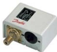
Danfoss KPI pressure switches are used for regulating, monitoring and alarm systems in industrial applications. The KP series are suitable for plant in connection with liquid and gaseous media. They are fitted with a single-pole switch changeover (SPDT).
