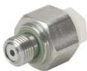
The MBV 2000 isolation valve is designed for mounting between a Danfoss pressure transmitter and fluid-filled systems and offers a fast and efficient method of connection and removal. The isolation valve automatically closes when a pressure transmitter is removed, so transmitters can be changed easily without having to first drain a system. The valve re-opens when a transmitter is connected. The valve meets demands for fast installation, simple and effective isolation and easy connection.
