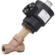
AV210 is an externally operated angle seat valve for use in robust industrial applications. The valve can operate at very high medium temperatures and viscosities, and is insensitive to dirt particles in the medium; thus, it is often called a "trouble-shooter" valve. The valve is available in gun metal (RG5/bronze) and stainless steel (AISI316).
