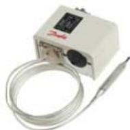
Danfoss KP thermostats are used for regulating, monitoring and alarm systems in industry. The KP series are temperature-operated electric circuit breakers. The thermostats are fitted with a single-pole switch (SPDT), and can control single-phase ac motors of up to 2 kW directly.
