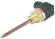
The MBT 3260 is a light duty temperature sensor that can be used for measuring and regulation in piping and ventilation systems and other light industrial applications. Due to the fact that the protection tube is made of copper the MBT 3260 has a very short response time of down to  $t_{0,5} = 2$  sec. in water. This temperature sensor is based on a standardized Pt100 or Pt1000 element, which gives a reliable and accurate measurement.
